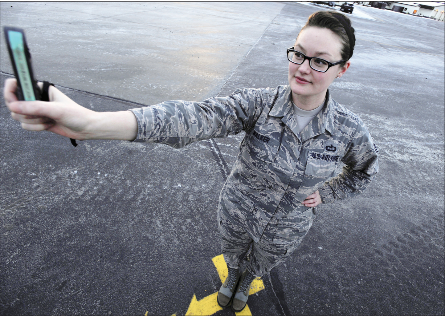
Air Force Staff Sgt. Dana Walker uses a kestrel meter to gauge wind and temperature readings from the official observing location, the most unobstructed view of the airfield, painted on the runway at Joint Base Elmendorf-Richardson, Alaska, Dec. 28. Walker is a weather forecaster assigned to the 3rd Operations Support Squadron. (U.S. Air Force photo/Staff Sgt. Robert Barnett)
