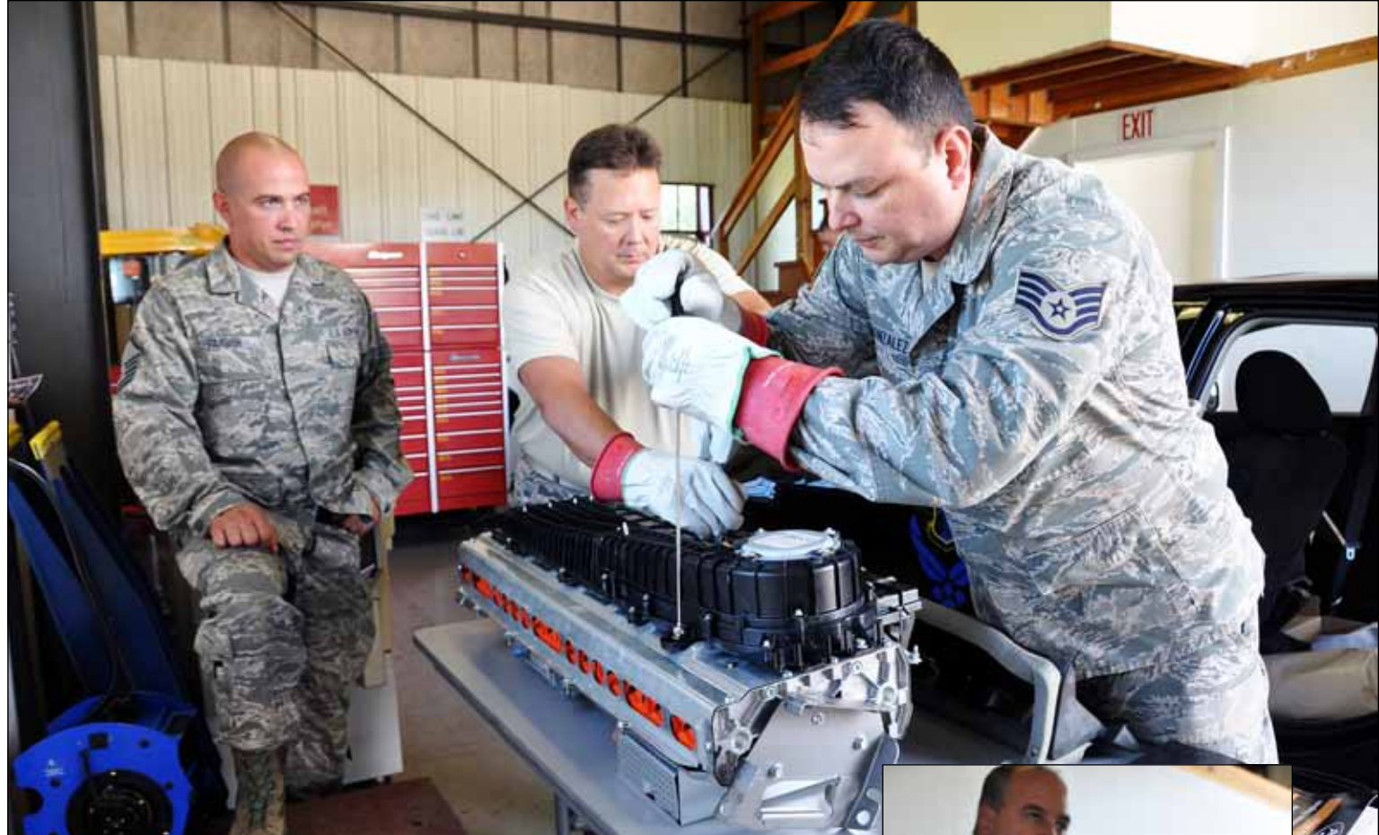
Above, Master Sgt. Tom Parrish, one of two hybrid vehicle maintenance instructors at Volk Field, observes as Master Sgt. Richard Witkowski and Staff Sgt. Manuel Gonzalez prepare a 275-volt battery back for reinstallation into a Ford Fusion hybrid car during an Aug. 27 class on hybrid vehicle maintenance. At right, Tech. Sgt. Tony Ortiz, of the Texas Air National Guard's 149th Fighter Wing, and Tech. Sgt. Scott Sweely, of the California Air National Guard's 165th Air Wing, reassemble electrical components. Wisconsin Department of Military Affairs photos by Vaughn R. Larson Click on image at right to see additional photos
