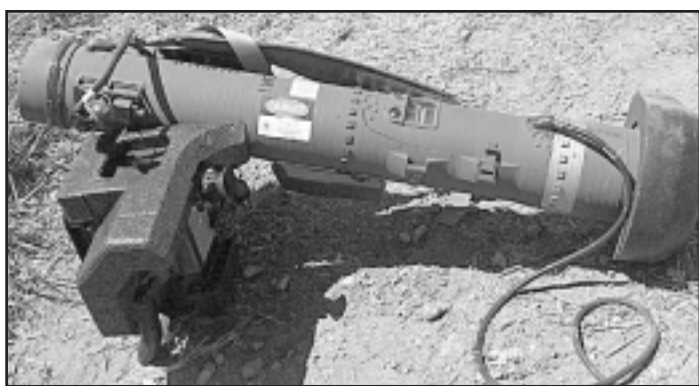
The M98 A-1 Javelin is a new missile system that Hawaii Marines are learning to operate, as well as the entire Marine Corps. This system can fire a missile that can track the movement of a target and then drops down on the target from above.
