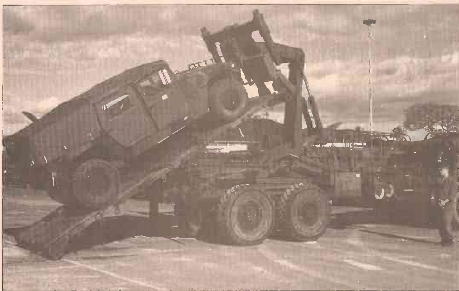
Lance Cpl. Joshua Karshner, a heavy truck operator for CSSG-3 Motor Transport Co., uses a remote control to load a "flatrack" and a humvee onto MK48/18A1.
