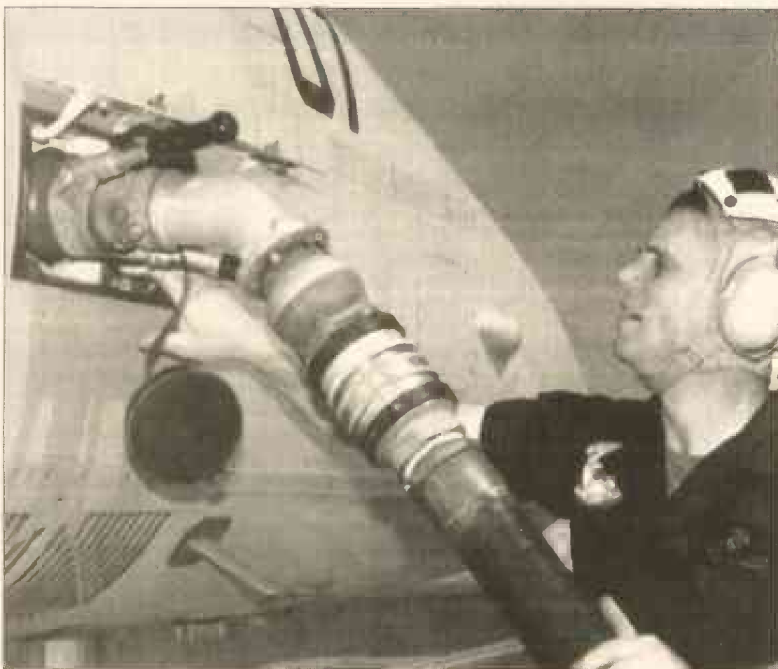
Sgt. Valerie Griffin Staff Sergeant David N. Hicks, safety staff noncommissioned officer in charge, Marine Fighter Attack Squadron 112, ensures fuel is flowing properly to an FA-18 Hornet during a hot refueling. Hot refueling is a Marine Corps specialty -- no other service conducts it.
