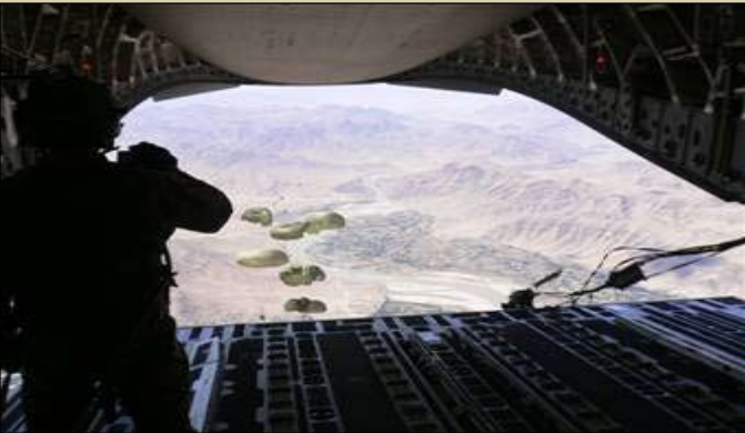
Staff Sgt. Derek Howard watches six container delivery system supply bundles as they parachute from a C-17 Globemaster III to the ground over Afghanistan May 24. The C-17 employed the Joint Precision Airdrop System in combination with the Improved Container Delivery System to increase accuracy of airdrops. (U.S. Air Force photo/Tech. Sgt. Gary Kleinfeldt)
