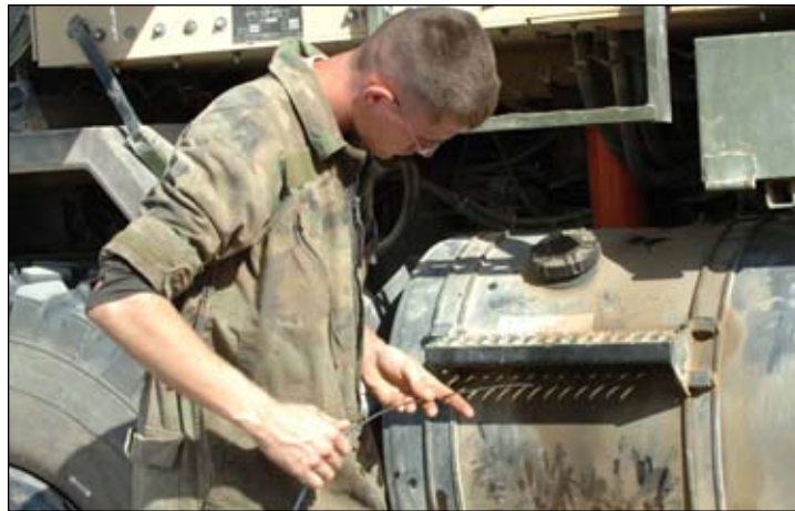
(Above) Spc. Andrew M. Nord, a mechanic with the 497th Transportation Company checks the oil of a heavy equipment transporter during a routine preventive maintenance checks and services. Nord is from Kansas City, Mo. (Below) Spc. Andrew M. Nord checks each tire of a heavy equipment transporter to see if they are flat or if they are missing any lug nuts, which could deadline the vehicle. (Bottom Left) Sgt. Louis Olvera, a palletized load list specialist from Davidson, Okla., 497th Transportation Company out of Fort Lewis, Wash., processes parts received from the SSA in Al Asad, Iraq.
