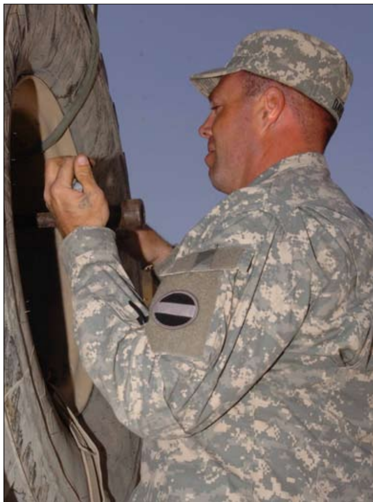
(Above) Pfc. Steffen Weiss, a wheeled mechanic, 497th Transportation Company out of Fort Lewis, Wash., changes the alternator belt on a heavy equipment transporter in Al Asad, Iraq. (Below) Staff Sgt. Travis J. Patterson, a shop foreman with the 497th Transportation Company updates a tracking sheet, which follows the status of vehicles returning from a mission outside the wire. Patterson is from Clinton, Iowa. (Left) Staff Sgt. Dusty A. Davis, senior wheeled vehicle operator, 497th Transportation Company, tightens the bolts of a palletized loading system. Davis is from Twin Falls, Idaho.
