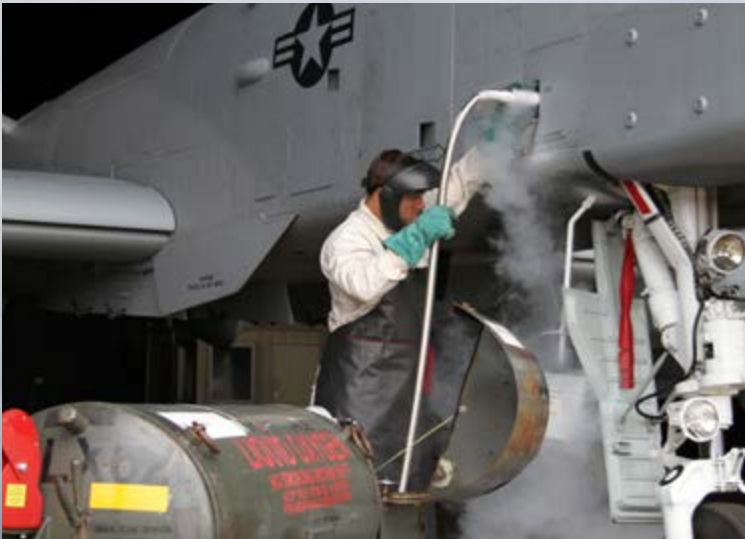
Senior Airman Ryan Keith of the 124th Maintenance Squadron, connects liquid oxygen service carts to provide oxygen to the A-10 Thunderbolt II pilots in flight during Operation Combined Resolve II.
