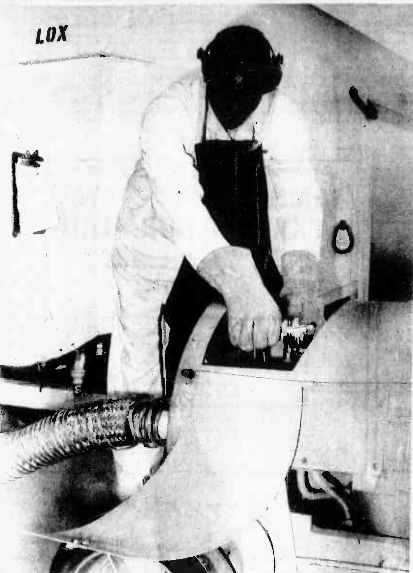
TIGHTENING DOWN — Corporal Robert Blanchard, cryogenics section, prepares to put a liquid oxygen sample in the infrared
