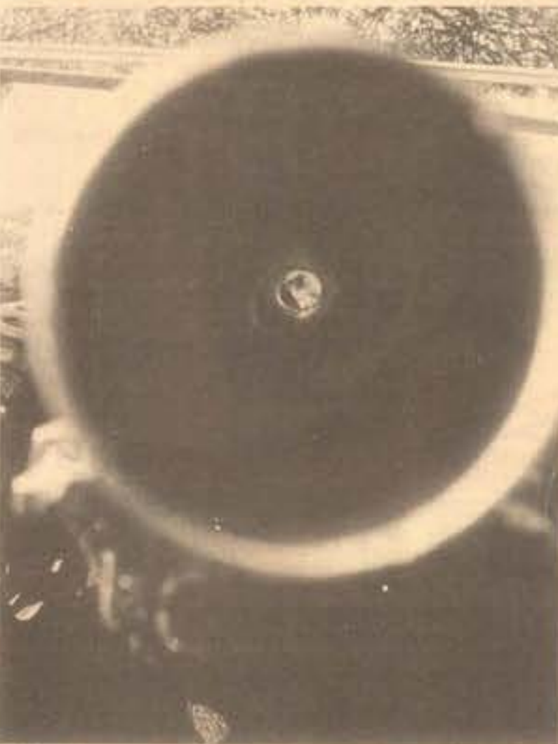
INSPECTING THE BORE — Private First Class Todd Foley, part of the 11-man detachment of the Fleet Marine Force, Pacific Saluting Battery, eyeballs the sides of the Pack 75mm howitzer's bore, making sure the interior is clean.
