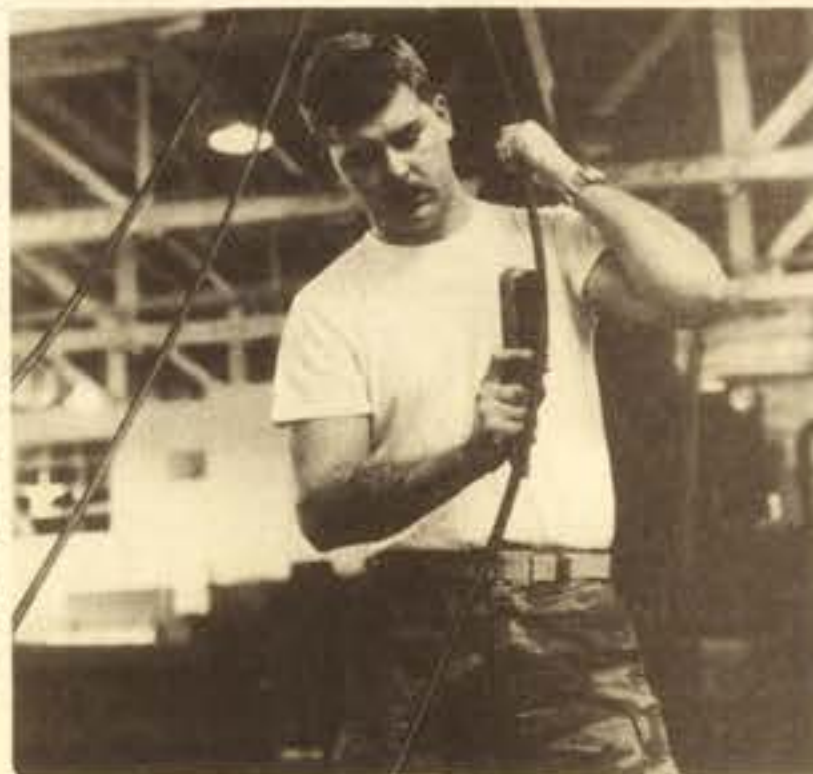
METICULOUS CARE — Sergeant Daniel Gay, maintenance shop chief, Marine Air Base Squadron-24, motor transportation, cleans a boom cable of a M-543 wrecker.
