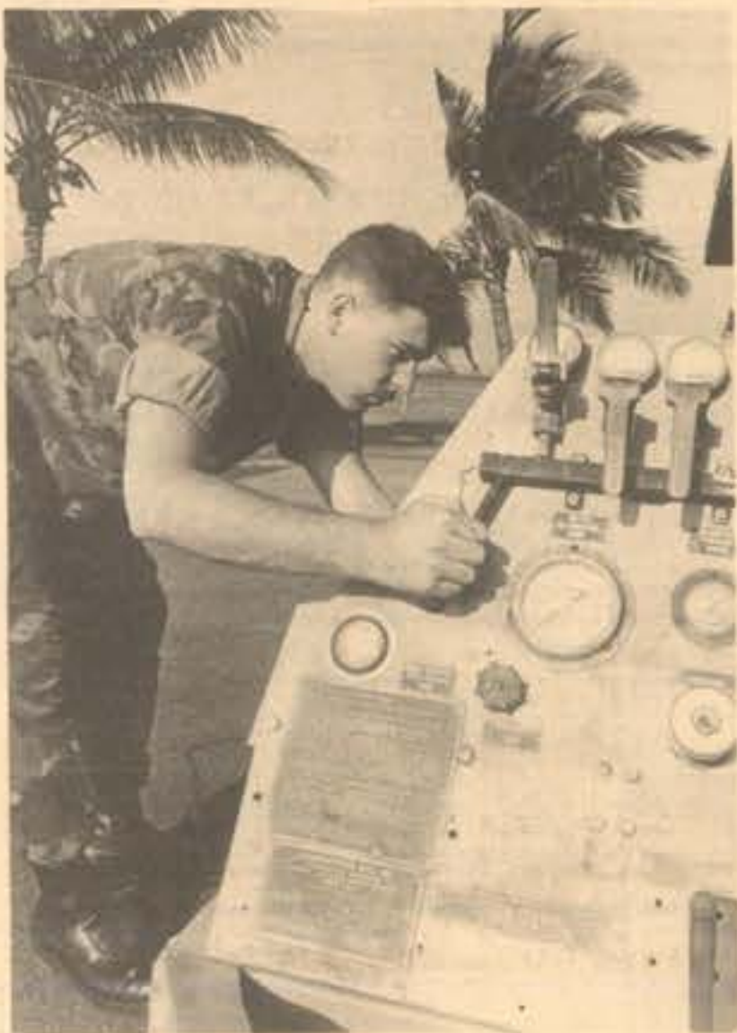
LOOKS GOOD — Private First Class Scott Barker, Cryogenics section, checks for pressure leaks in tanks fastened to the back of a nitrogen cart. The nitrogen cart is used for charging hydraulic systems in aircraft.
