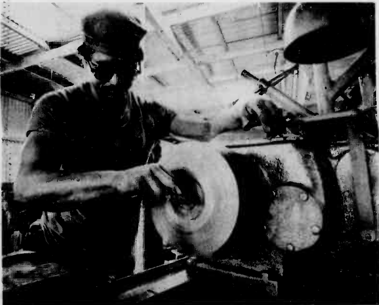
HEAVY METAL — Mitchell Au, heavy equipment mechanic, grinds an engine valve stem. Au is one of 36 civilian
