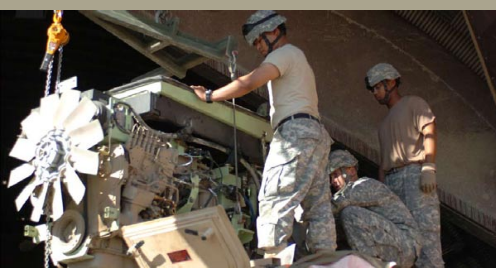
In the final day of the 40-hour course, Soldiers reinstall an engine in an M1117 Guardian Armored Security Vehicle.
