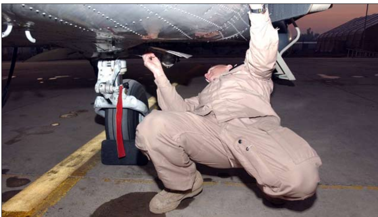
Staff Sgt. Edwin Agregaard checks the landing gear of the C-23 Sherpa aircraft during his preflight checks. The flight engineer must check every part of the plane for cracks and defects which could cause problems while in flight.
