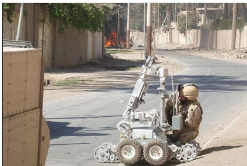
Senior Airman Kyle Preece, 332nd Expeditionary Civil Engineer Squadron Explosive Ordnance Disposal Flight, works on the F6A robot as a vehicle borne improvised explosive device burns in the background.
