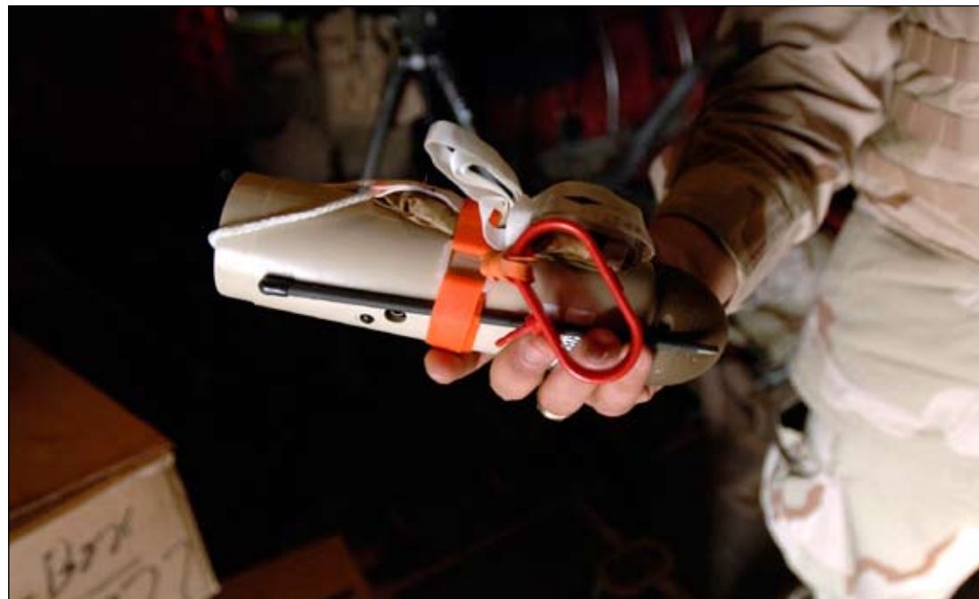
An airman holds a wind sonde device that is dropped at high altitudes over a drop zone to measure the winds prior to an actual cargo drop. This allows C-130 crews to drop cargo at safe distances from enemy fire. This one was used during an OIF drop somewhere in the skies of Iraq.
