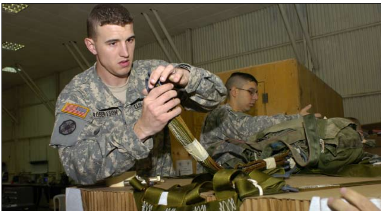
Spc. James Robertson, assigned to the 600th Quartermaster Detachment, attaches the suspension risers to a parachute. This link that holds the load to the parachute.
