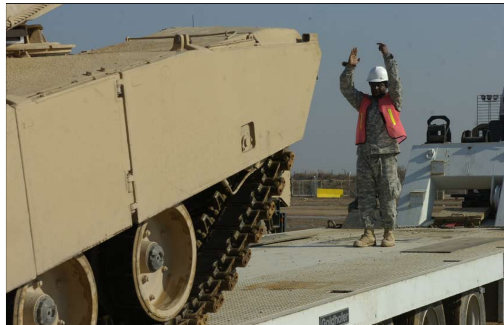
Sgt. Calvin Edwards, a transportation management coordinator from Chicago, Ill., carefully guides an M1A1 Abrams Main Battle Tank onto a truck.
