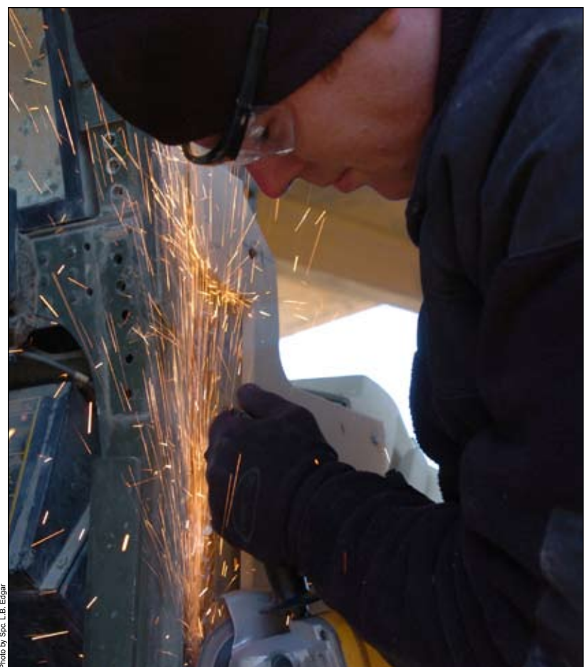
Photo by Spc. L.B. Edgar Spc. Robert Maloney, heater and air conditioner repair mechanic, 289th Quartermaster Company, grinds down the door frame of a Humvee at the Baghdad International Airport Vehicle Enhancement Site, Iraq.
