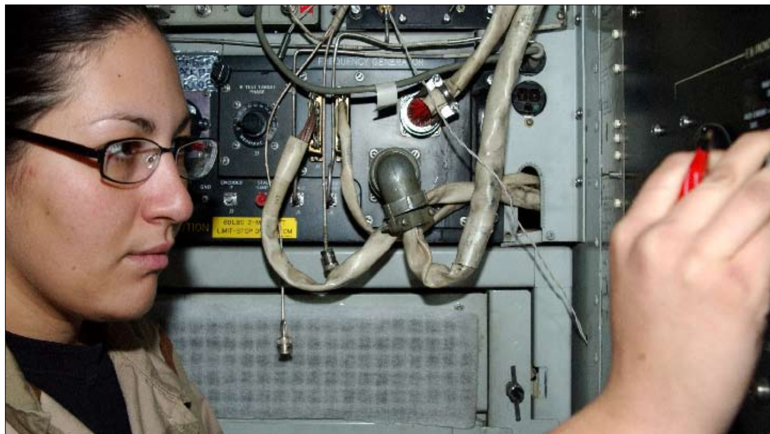
Senior Airman Adrienne Samora conducts a daily preventative maintenance inspection Dec. 19 on one of the ground radar systems at Balad Air Base, Iraq. Airman Samora, a 727th Expeditionary Air Control Squadron radar maintenance technician, is deployed from Mountain Home Air Force Base, Idaho.
