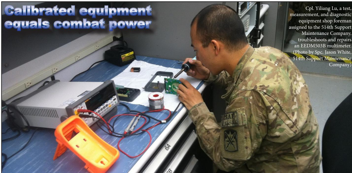
Cpl. Yiliang Lu, a test, measurement, and diagnostic equipment shop foreman assigned to the 514th Support Maintenance Company, troubleshoots and repairs an EEDM503B multimeter. (Photo by Spc. Jason White, 514th Support Maintenance Company)
