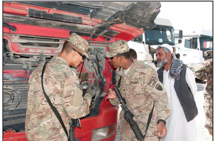
Spc. Keshab Ghosh, right, a gunner assigned to 730th Transportation Company, checks the oil level of a host nation truck to ensure it is mission capable. Soldiers also checked fuel levels, tire tread and batteries to minimize maintenance issues they may have encountered during the mission. (Photo by Sgt. 1st Class Luis Saavedra, 10th Sustainment Brigade PAO)
