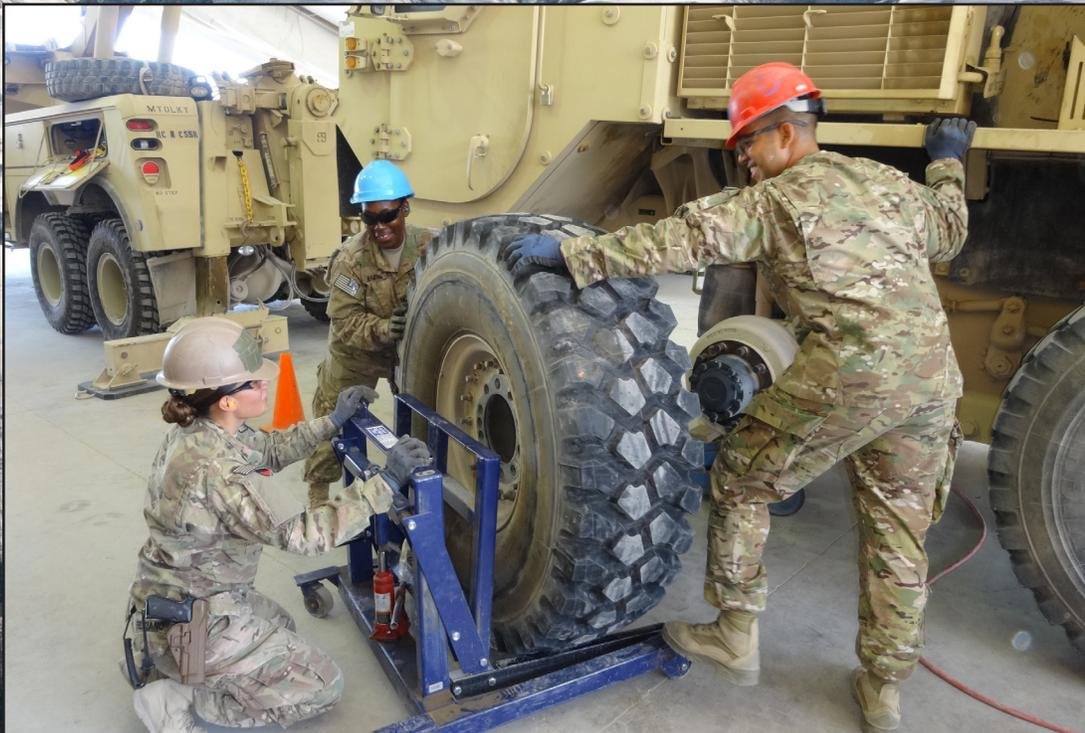
Two maintenance Soldiers assigned to the 1569th Transportation Company, provide instructions to 2nd Lt. Alexandra Feliciano on the proper procedures to replace a tire on a heavy expanded mobility tactical truck with a load handling system. (Courtesy Photo)
