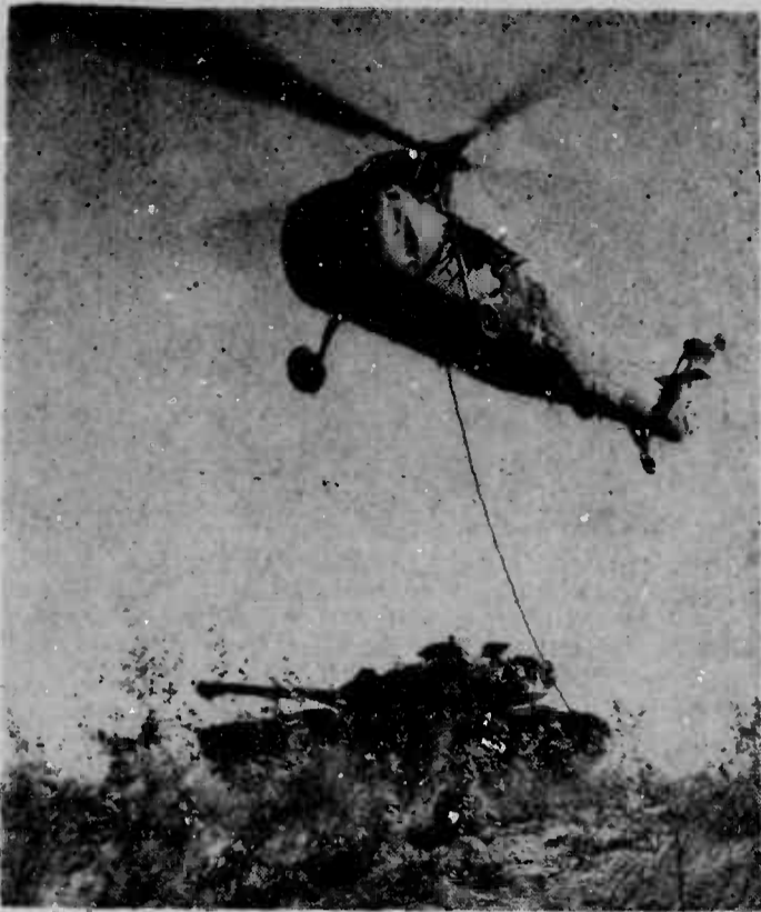
FLYING GAS STATION — While operating "in the field," an infantry tank replenished its fuel supply via a tanker helicopter hovering less than 30 feet overhead. Both Marine Corps vehicles combined their efforts to test another milestone in aviation history — Air-to-ground refueling.
