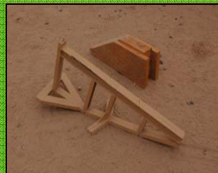
A photo of the two-piece, ‘Patriot Jack,’ assembly. The device has helped dozens of soldiers with changing tires while on dangerous missions.
