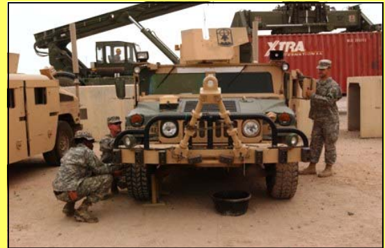
Soldiers of the 121 Field Artillery Battery demonstrate the, “Patriot Jack,” a recent invention to assist convoy security teams with changing tires while on missions in Iraq.
