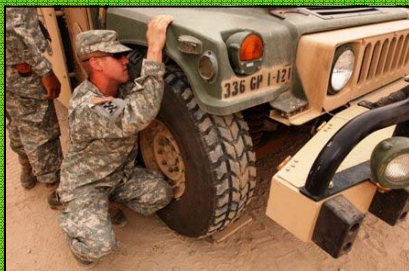
Sgt. Andrew Plier, a light-wheel mechanic for the 121 FA—Maintenance Section adjusts part of the jack assembly during a demonstration under an M114 HMMWV.
