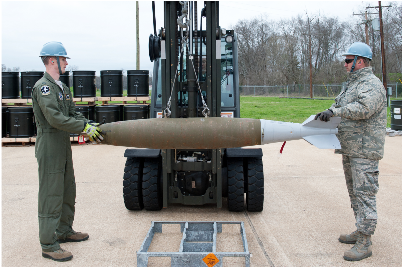
1st Lt. Mike Binford, 190th Fighter Wing "Warthog" pilot, left, with Senior Airman Craig Hereau, 124th Maintenance Squadron, Munitions Flight, built a MK 82 low-drag bomb, that 1st Lt. Binford then loaded, secured, safety checked, autographed with his call sign, and dropped the 500 pound bomb from the A-10 Thunderbolt II aircraft on March 16 at Barksdale Air Force Base, La. (Air National Guard photo by Master Sgt. Becky Vanshur)
