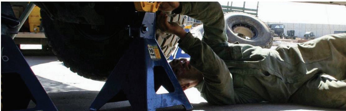
Pvt. Juan Tajeda, 2-6 Cav., E Troop, light wheel vehicle mechanic, places a jack stand under a humvee as the service crew prepares to check the wheel bearings at FOB Warrior, Kirkurk Iraq.
