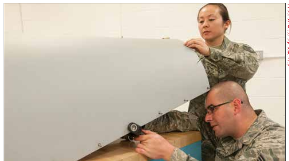
Tech. Sgt. Erika Serrano and Senior Airman Leonard Enciso of the 163rd Reconnaissance Wing Maintenance Group perform structural maintenance on an MQ-1 Predator remotely piloted aircraft Nov. 4 on March Air Reserve Base in Riverside, Calif.
