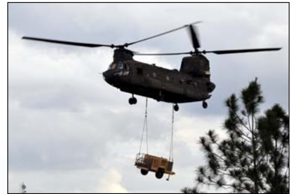
A CH-47 Chinook helicopter assigned to the 1-228th Aviation Regiment approaches Mocomon, Honduras, while carrying a sling-loaded generator in order to set up a tactical operating base for a Collective Training Exercise Nov. 18
