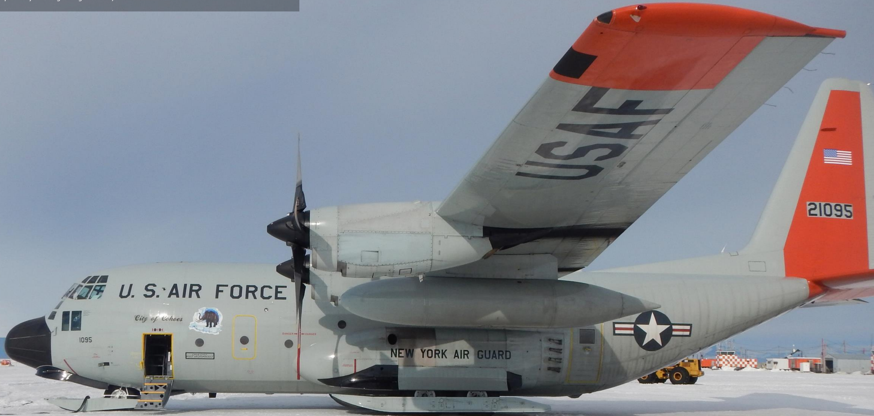
An LC-130 Hercules from the New York Air National Guard's 109th Airlift Wing transports cargo on Antarctica. Note the special skis that the aircraft uses for takeoff and landing. (U.S. Air National Guard photo by Tech. Sgt. Greg Mascaro)
