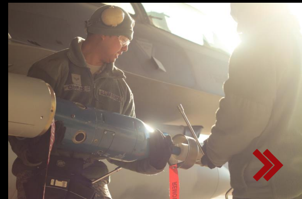
Above: U.S. Air Force Senior Airman James Mullen from the New Jersey Air National Guard's 177th Fighter Wing assembles fins on a GBU-12 Paveway II mounted on an F-16C Fighting Falcon during day one of the annual load crew competition here on Jan. 9. Below: U.S. Air Force Airman 1st Class Desmond Charles from the New Jersey Air National Guard's 177th Fighter Wing unloads the computer control group from a GBU-12 Paveway II on Jan. 9. Charles is a weapons systems specialist from the 177th Aircraft Maintenance Squadron. (U.S. Air National Guard photos by Tech. Sgt. Matt Hecht)
