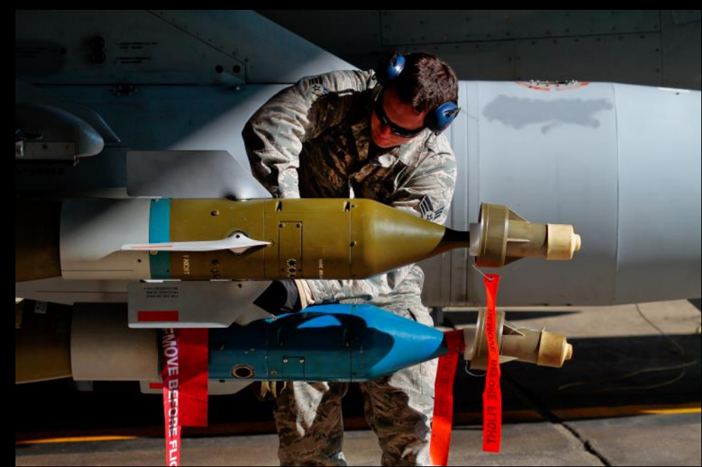
Above: U.S. Air Force Senior Airman James Mullen from the New Jersey Air National Guard's 177th Fighter Wing assembles fins on a GBU-12 Paveway II mounted on an F-16C Fighting Falcon during day one of the annual load crew competition here on Jan. 9. Below: U.S. Air Force Airman 1st Class Desmond Charles from the New Jersey Air National Guard's 177th Fighter Wing unloads the computer control group from a GBU-12 Paveway II on Jan. 9. Charles is a weapons systems specialist from the 177th Aircraft Maintenance Squadron. (U.S. Air National Guard photos by Tech. Sgt. Matt Hecht)
