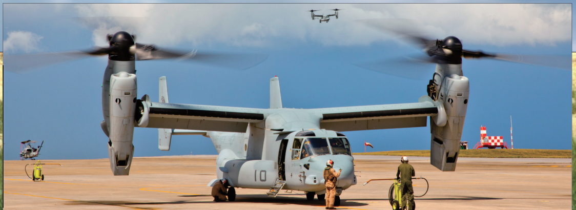
MV-22B Osprey tiltrotor aircraft land at Marine Corps Air Station Futenma Aug. 12 after flying from MCAS Iwakuni. The tiltrotor aircraft combines the vertical capability of a helicopter with the speed and range of a fixed-wing aircraft, enabling it to fly twice as fast, carry three times as much, and fly four times the distance of the older CH-46Es it replaced. The Ospreys and crews are assigned to VMM-262. Photo by Lance Cpl. Stephen Himes
