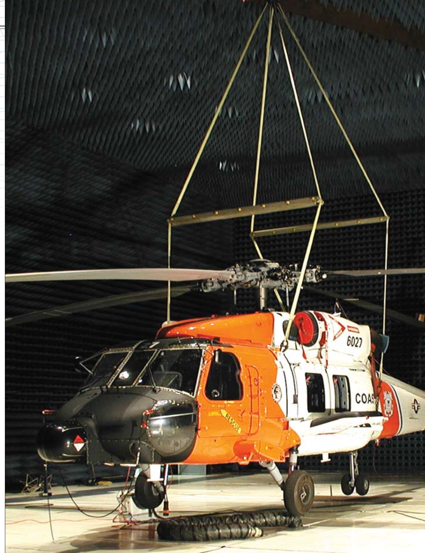
↑ JAZZED-UP JAYHAWK An HH-60 Jayhawk Medium Range Recovery helicopter undergoes testing at Patuxent River, Md., Sept. 19, 2007, as part of the conversion process into the MH-60J/T, a modification to meet Airborne Use of Force requirements. The Medium Range Recovery program represents one of the most comprehensive aviation upgrade programs in Coast Guard history. The Coast Guard’s MRR program will deliver a total of 42 MH-60T configured aircraft for Coast Guard operations.
