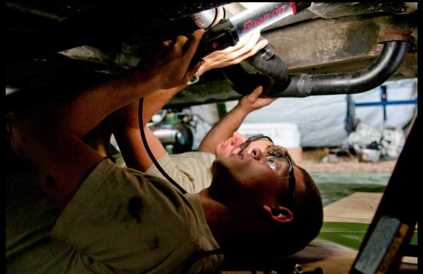
BELOW: U.S. Army Spc. Taylor Gingras and Pvt. Nicholas Amature, with Bravo Company, 186th BSB, replace a Y-pipe on a truck while training at Fort Drum, N.Y., Aug. 7, 2013. The 86th IBCT is conducting their XCTC in preparation for their rotation at the Joint Readiness Training Center. (U.S. Air National Guard photo by Staff Sgt. Sarah Mattison)
