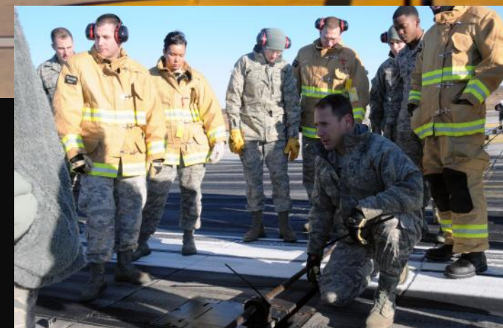
Master Sgt. Bruno Egizi from the 177th Civil Engineering Squadron Fire Department instructs airmen during a test of the runway aircraft arrest system Nov. 14 at the 177th Fighter Wing at Atlantic City Air National Guard Base, N.J. The arrest system is used to stop aircraft in the event of a brake failure and must be tested yearly. (U.S. Air National Guard photo by Airman First Class Shane Karp)
