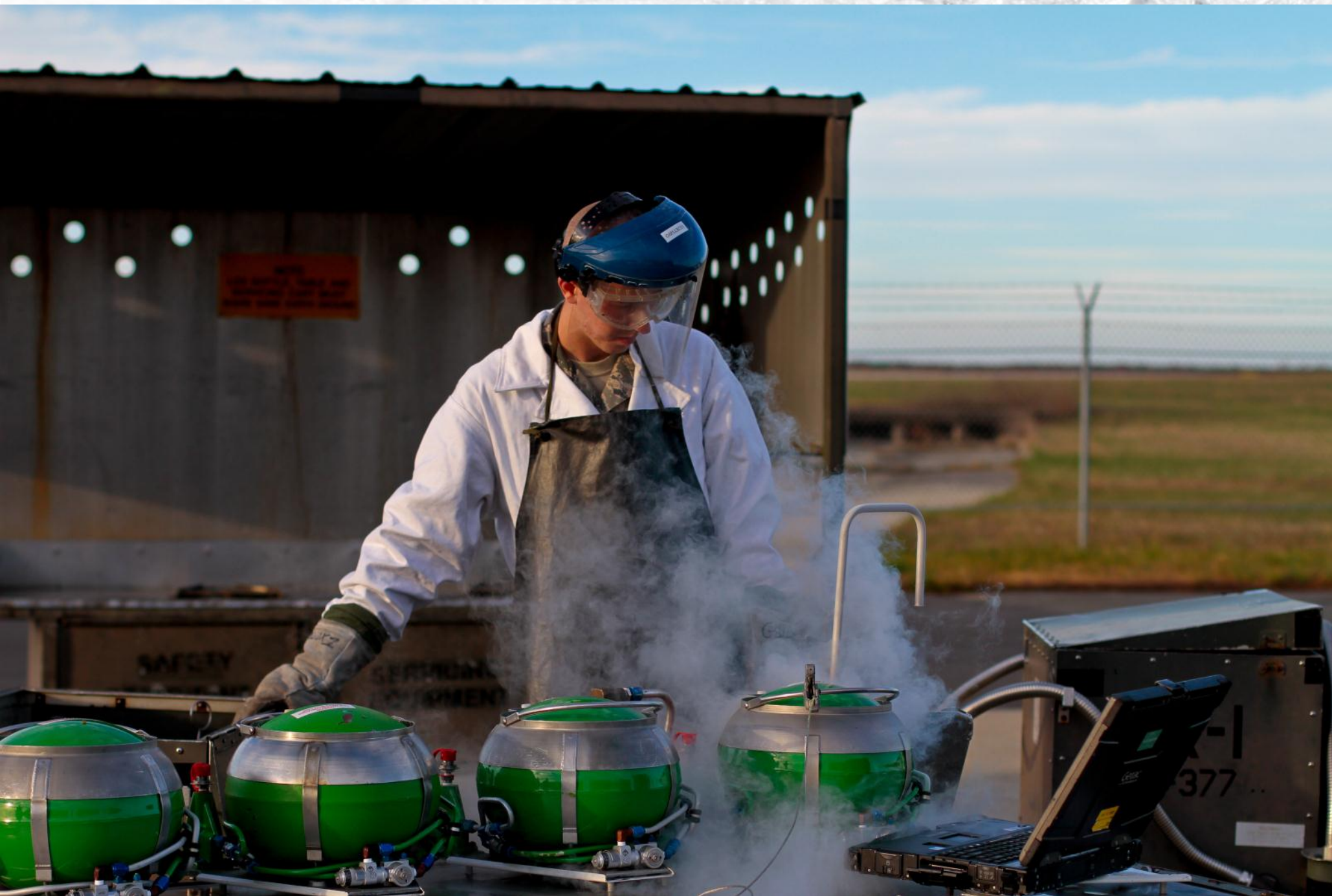
Airman 1st Class Christopher Garrison performs Liquid Oxygen (LOX) servicing at Atlantic City Air National Guard Base, N.J. on Nov. 6. LOX is primarily used as aviator breathing oxygen. Garrison is an F-16C Fighting Falcon crew chief assigned to the 177th Aircraft Maintenance Squadron.
