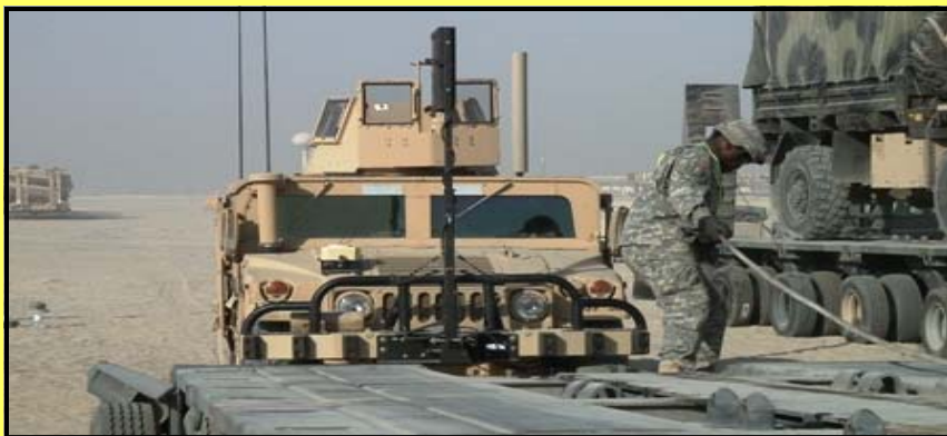
A Soldier pulls down a cable to hitch and tow a vehicle onto the flatbed of a Heavy Equipment Transporter truck, during a training exercise on convoy vehicles and operations. The 1st Battalion, 77th Heavy Equipment Transporter Company trained the 217th Transportation Company in Kuwait for future missions into Iraq.
