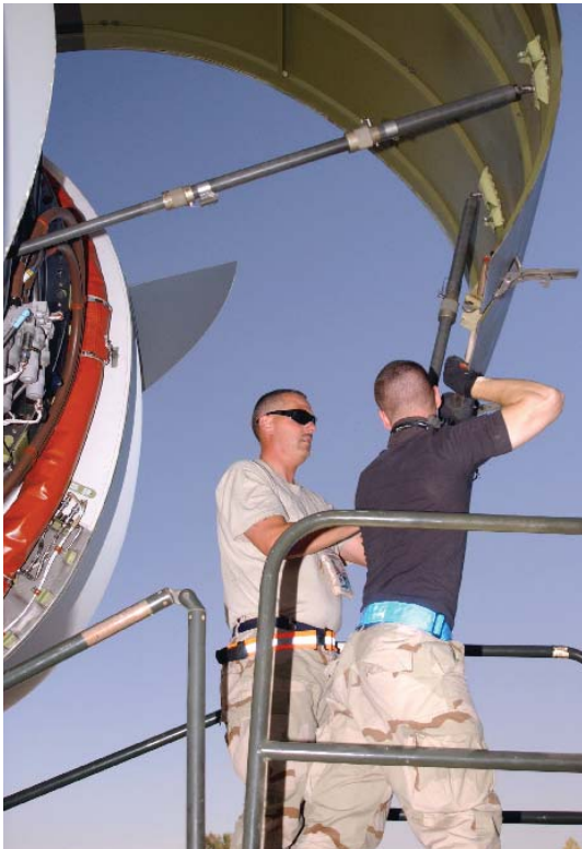
Staff Sgt. Robert Miller and Airman 1st Class Mark Mano, 721st Air Mobility Operations Group, Detachment 5, open the engine cowl of a C-17 Globemaster on Tuesday.
