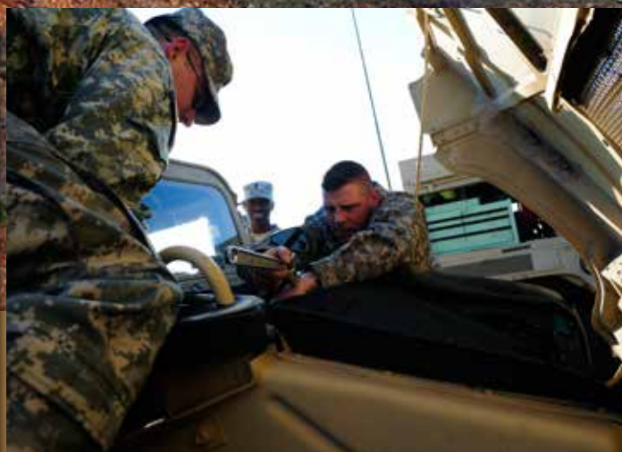
Soldiers from the 31st Air Defense Artillery Brigade, 3rd Battalion, 2nd Air Defense Artillery Regiment, repair a leak on the power steering system of a Humvee Jan. 14, 2013.
