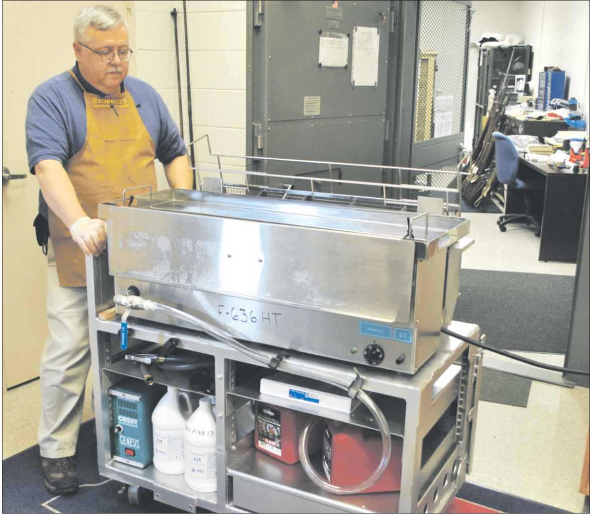
MAFM Arms Conservator Glenn Husted stands next to the Crest Ultrasonic Cleaning System during the treatment of weapons parts in the Arms Conservatory.
