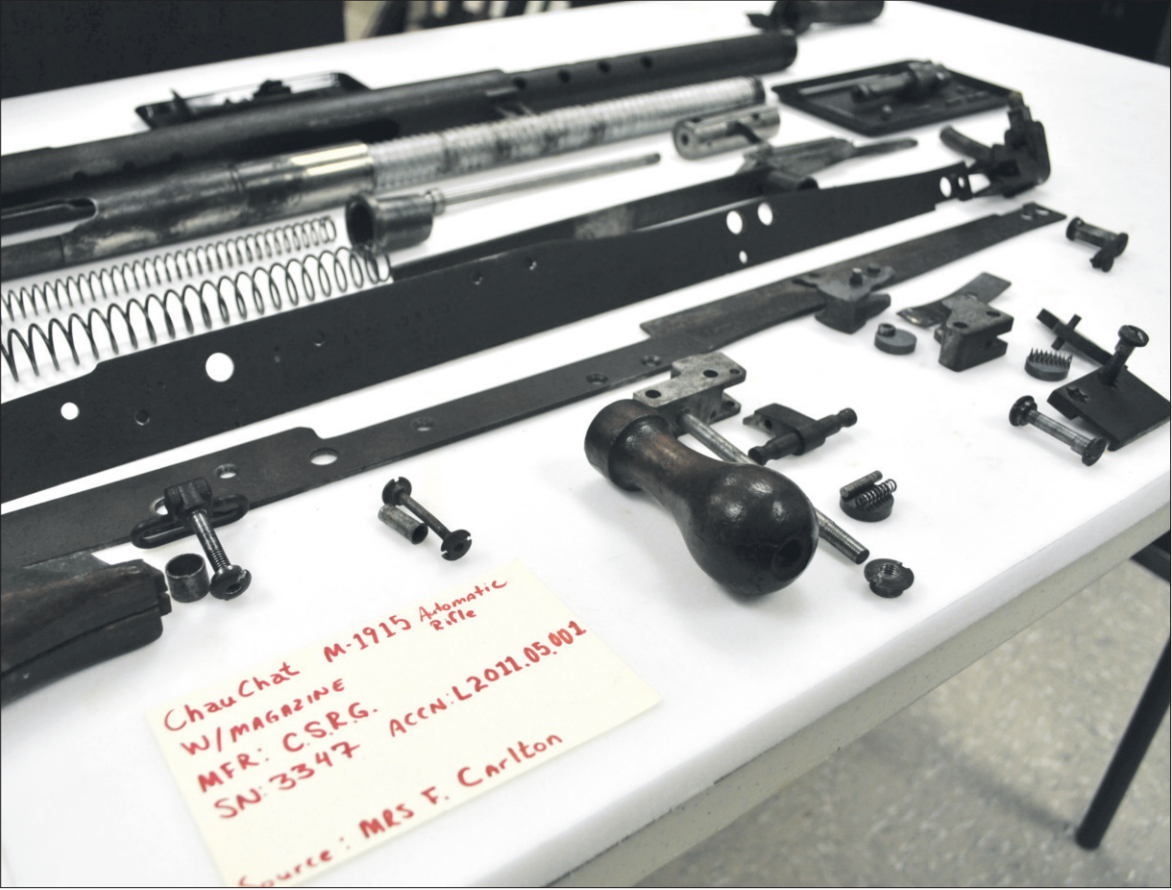
A fully disassembled M-1915 Chauchat automatic rifle waits to be immersed in the ultrasonic cleaner as part of the preservation process at the museum.
