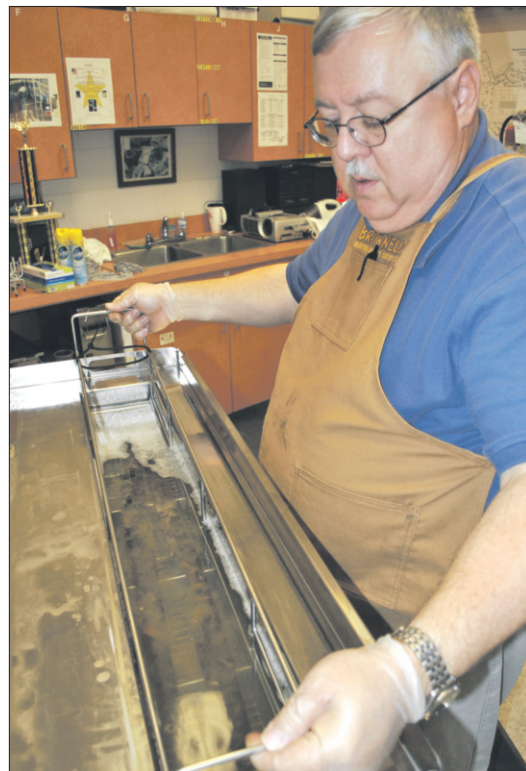
From left, Arms Conservator Glenn Husted and Museum Volunteer Tim McGuyer pre-clean parts of an M-1915 Chauchat automatic rifle before immersing them in the ultrasonic cleaning system. Below, Husted slowly immerses parts of an M-1915 Chauchat automatic rifle into the ultrasonic cleaning system, where rust and oil are already blooming off the submerged parts.
