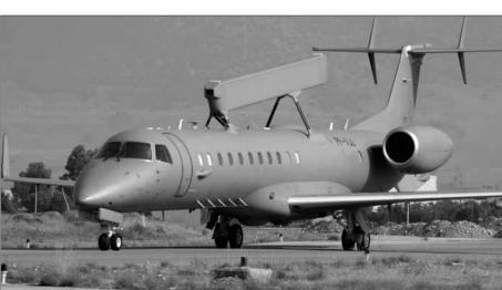
The PSR (PS 890) manufactured by Ericsson, is an electronically scanned array multi-mode long-range radar. It processes the acquired air and maritime surveillance information in Real -Time to the C2 (Command and Control) system. The dorsal-mounted antenna is flat and lightweight, so it produces low aerodynamic drag.
