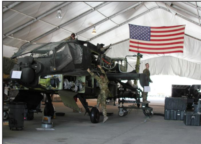
**AH-64 Apache helicopter maintenance Soldiers assigned to D Company, 1st Attack/Reconnaissance Battalion, 501st Aviation Regiment, Task Force Dragon, inspect for deficiencies during a 500-hour phase maintenance inspection June 27, at Forward Operating Base Fenty. (Photo by Sgt. Armando Avila, Task Force Dragon)**
