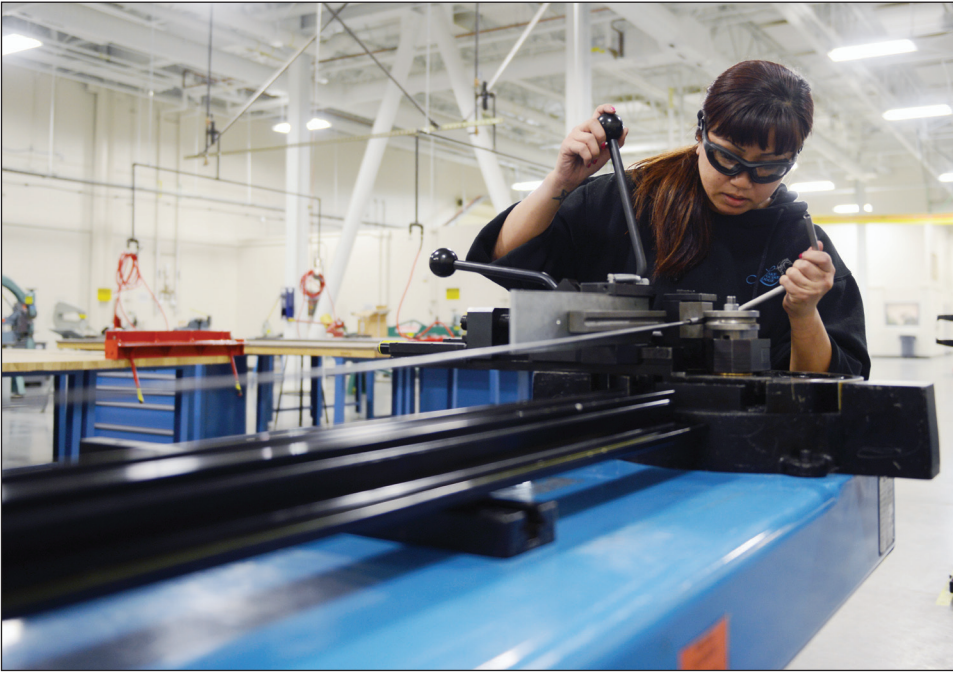
Janny Dunlavey, aircraft structural maintenance craftsman with the 3rd Maintenance Squadron uses a tube bender to manufacture hydraulic lines for an aircraft at the Aircraft Structural Maintenance shop March 25. A critical aspect of the Aircraft Structural Maintenance Shop is to take damaged aircraft materials and refurbish them to thier original hull integrity. (U.S. Air Force photo/Airman Ty-Rico Lea)
