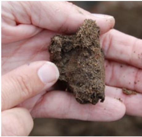
Iron depletion (seen as the rusty orange color) is a redoximorphic feature used to identify hydric soils. During field investigations, biologists look for identifiers such as these to help determine whether to classify an area as a wetland. (Photo by Greg Fuderer)
