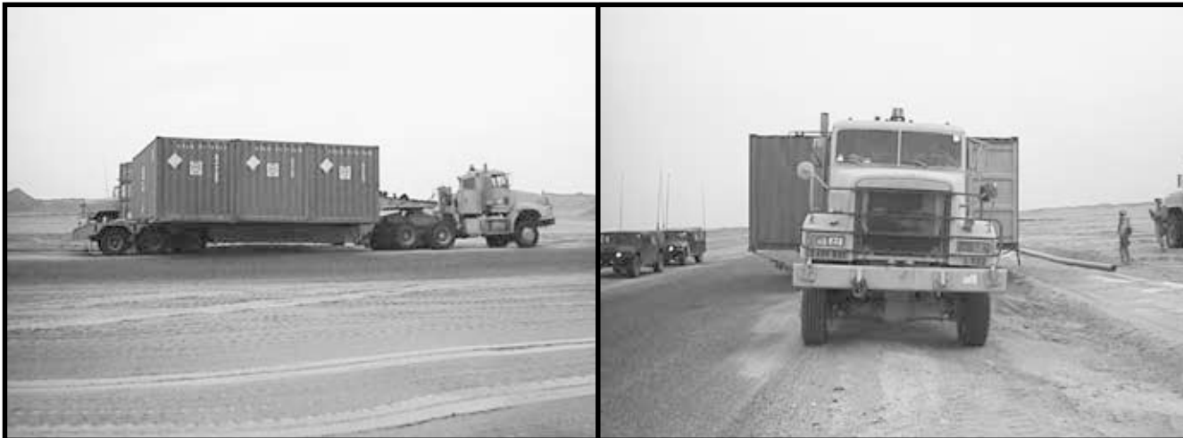
Alpha Company, 62d Engineer Battalion, transports pipe by loading three MILVANs on a lowboy.
