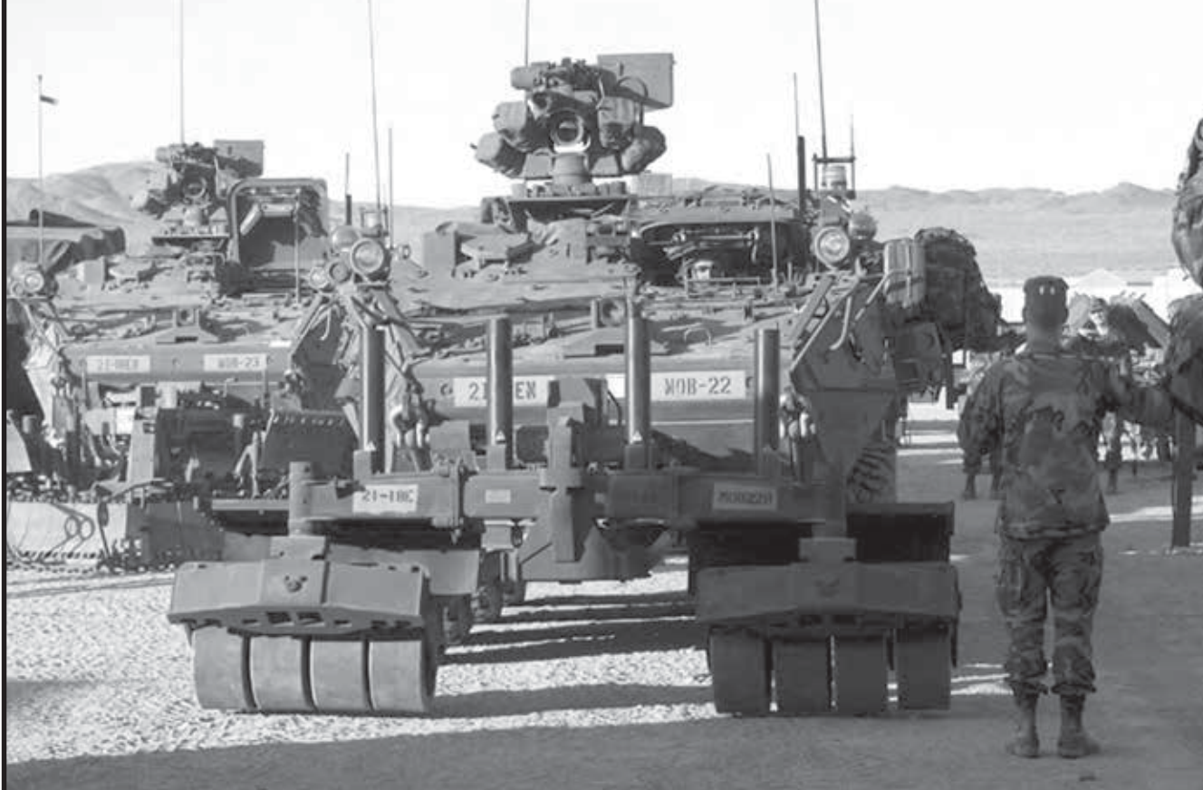
The ESV can be outfitted with a mine plow (left) or a mine roller (right).
