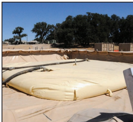
This bladder is used to store fuel until it is distributed. The bladder can hold up to 20,000 gallons of fuel. Soldiers with the 728th and 192nd Quartermaster Companies were responsible for bulk and retail fuel at Fort Hunter Liggett, Calif., for Combat Support Training Exercise 91.
