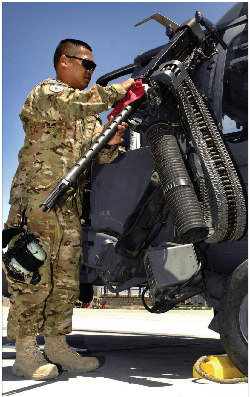
U.S. Air Force Tech. Sgt. John Arquitola, 33rd Expeditionary Helicopter Maintenance Unit HH-60G Pave Hawk weapons section expeditor, inspects and cleans a mounted .50-caliber machine gun on a U.S. Air Force HH-60G Pave Hawk helicopter at Bagram Air Field May 24. Arquitola, a resident of Keaau, Hawaii, is part of a team of crew members that check the HH-60Gs to make sure all parts are in place and secure, and that the weapons systems are serviceable. (Photo by U.S. Air Force Staff Sgt. Jeff Nevison)
