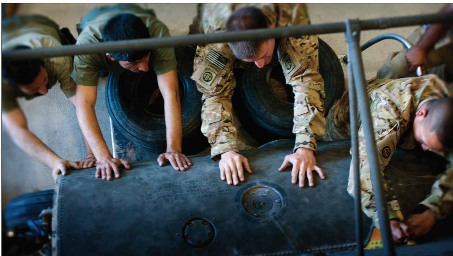
U.S. Army Sgt. Christopher Burr, of Virginia Beach, Va., and Pvt. Felix Reyes, of Chicago, both of the 122nd Aviation Support Battalion, 82nd Combat Aviation Brigade, remove an auxiliary fuel tank from a CH-47 Chinook helicopter with the help of Afghan 1st Lt. Asif Wahidi and Afghan 1st Lt. Mohammed-Ullah Kohdamani from the Afghan Ministry of the Interior Special Missions Wing June 9. The U.S.-Afghan partnership is part of a program designed to share aviation maintenance techniques and safety procedures between the two units. (Photo by U.S. Army Sgt. 1st Class Eric Pahon, TF 1-82 PAO)
