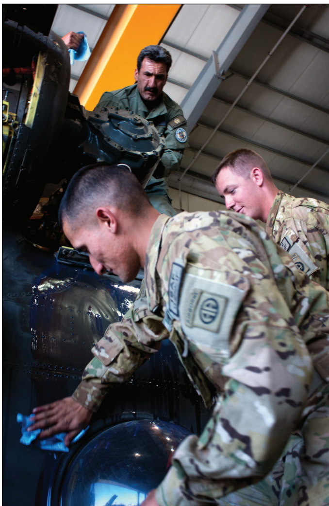
U.S. Army Spc. Israel Vela, a native of Houston and an aviation mechanic with 122nd Aviation Support Battalion, 82nd Combat Aviation Brigade, wipes hydraulic fluid from the side of a CH-47D June 9. Vela, U.S. Army Spc. Jessie Wentworth, of Hesperia, Calif., and Afghan Sgt. Said Iqbal, an aviation mechanic from the Afghan Ministry of the Interior Special Missions Wing worked together during a new U.S.-Afghan partnership training program designed to share U.S. aircraft maintenance techniques and safety practices with Afghan counterparts. (Photo by U.S. Army Sgt. 1st Class Eric Pahon, TF 1-82 PAO)
