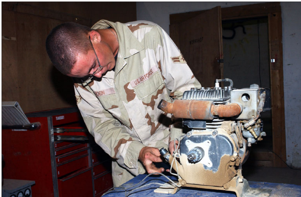
Airman 1st Class Andrew Moen, 407th Expeditionary Operations Support Squadron, maintains a two-cycle engine from a portable heater. (Photos by Master Sgt. Andrew Gates)
