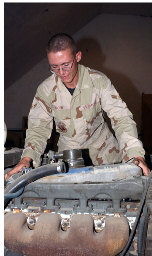
Airman Moen removes the valve cover from a Dash-86 diesel generator during a tune up.
