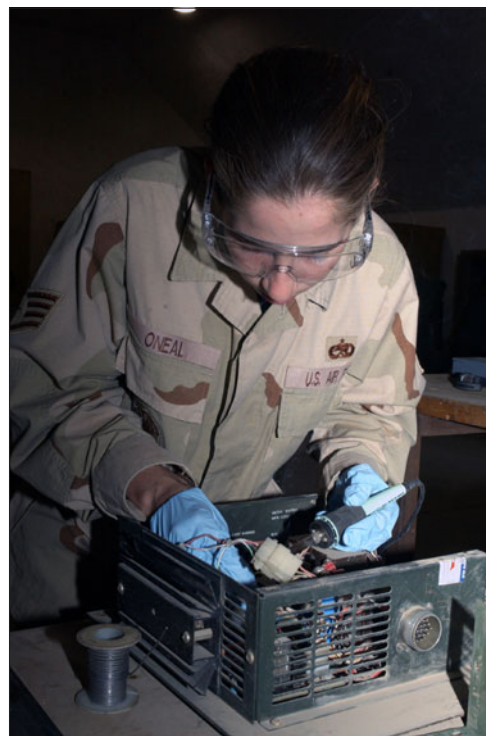
Staff Sgt. Jacquelin O'Neal, 407th EOSS, solders a voltage regulator for a Dash-86 generator.
