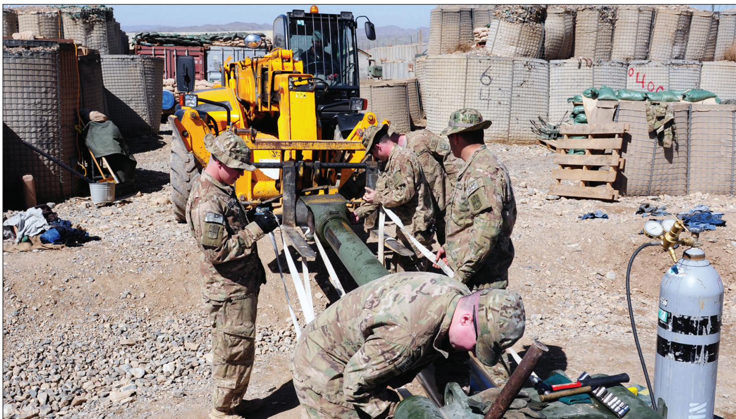
Artillerymen with 1st Battalion, 172nd Infantry Brigade, Task Force Blackhawk use a forklift to depress the muzzle of an M777A2 155mm Howitzer at Forward Operating Base Boris March 5. Once they depress the muzzle, they can inspect the breech more thoroughly. (U.S. Army photo by Sgt. William Begley, RC-East PAO)
