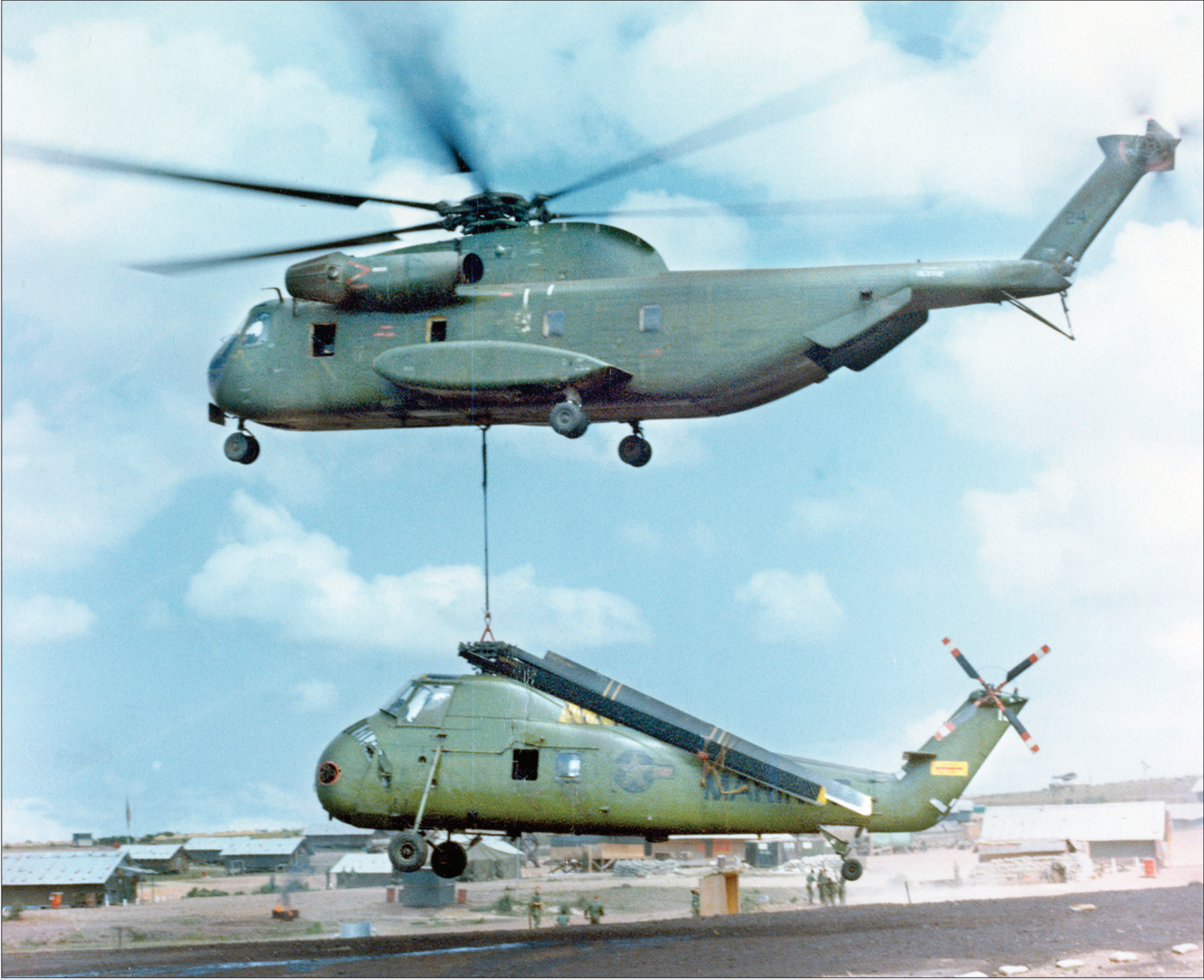
A CH-53A lifts a UH-34D in Vietnam. The Stallions have been serving in the Marine Corps since 1967 as a heavy assault helicopter developed by Sikorsky. It is often regarded as one of the largest and most powerful helicopters in the world.
