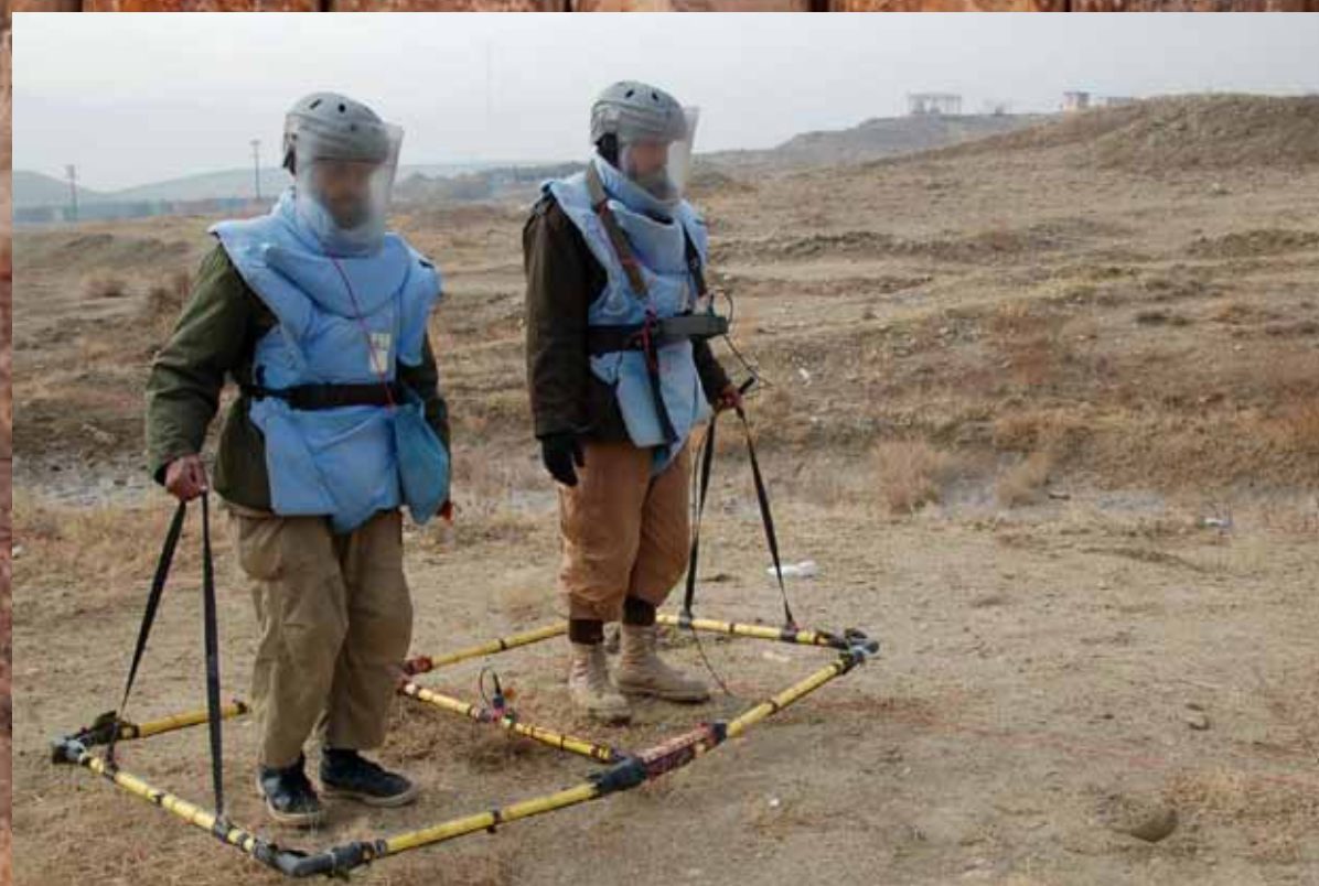
Ronco De-mining contractors use deep Ebinger Large Loop Detector to find unexploded ordnance. Ground must be cleared to a depth of one meter to fulfill de-mining specifications. (Photo by Hank Heusinkveld)
