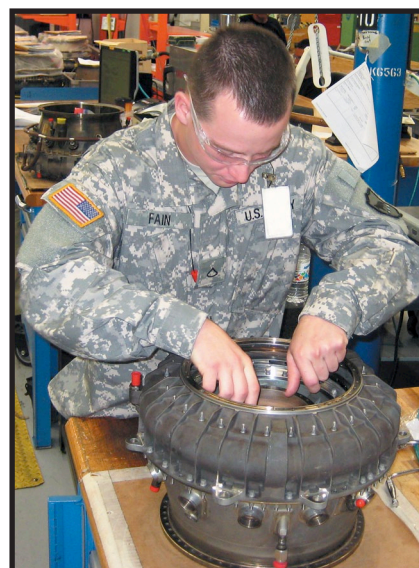
Pfc. Jacob P. Fain, Det. I, Co. B, 935th Support Battalion, re-assembles a hot-section for a T700 engine for a UH-60 helicopter, during annual training at the Corpus Christi Army Depot in Corpus Christi, Texas.
