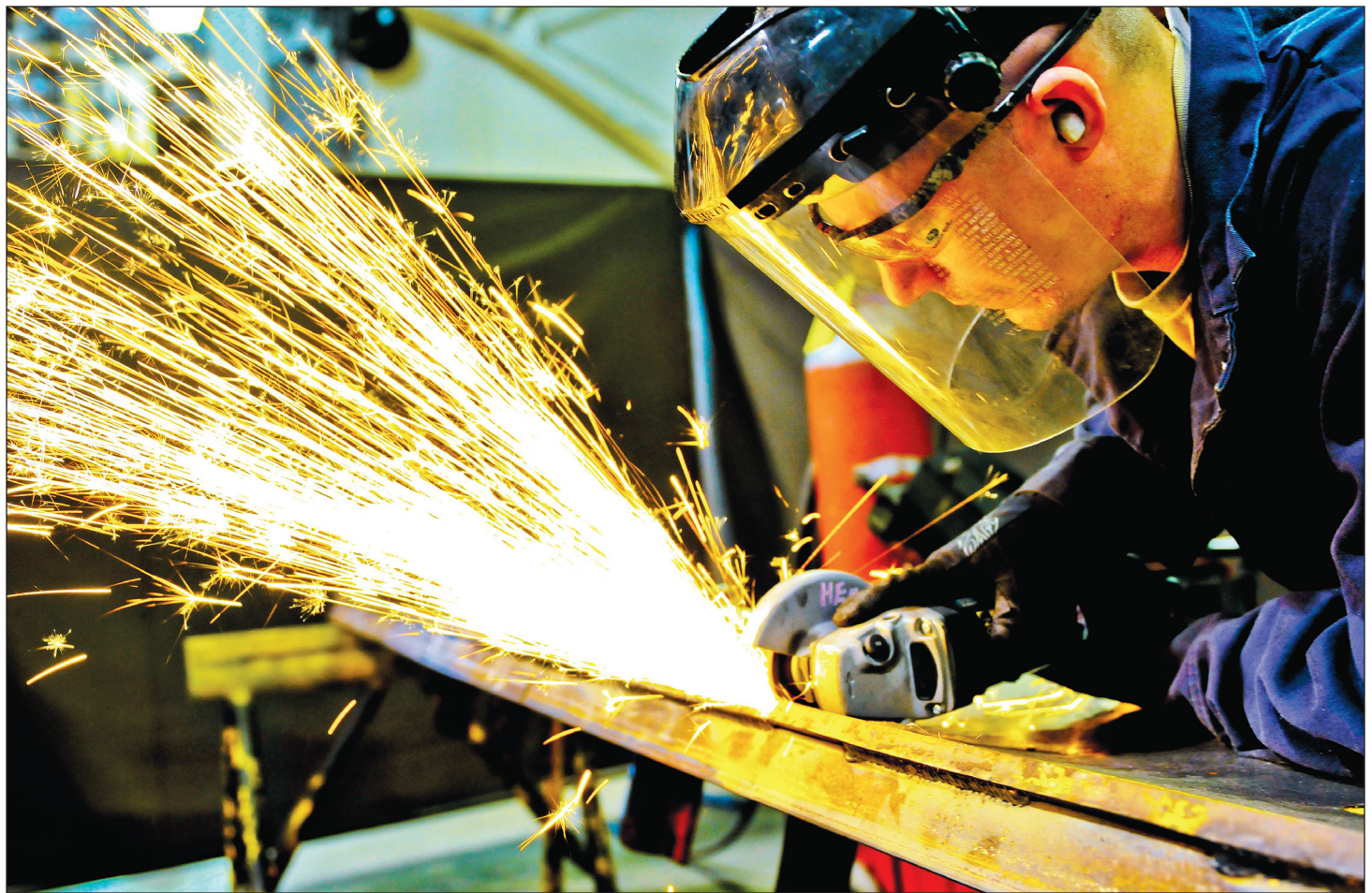
Senior Airman Shane Harrington, 673d Logistics Readiness Squadron, grinds down a crack in a snow plow, Sept. 28, before repairing the crack with a weld. The 673d Logistics Readiness Group earned an outstanding rating – the highest mark – during a Logistics Compliance Assessment Program inspection administered by Air Combat Command, Joint Base Langley-Eustis, Va., and Pacific Air Forces, Joint Base Pearl Harbor-Hickam, Hawaii. (U.S. Air Force photo/Steve White)
