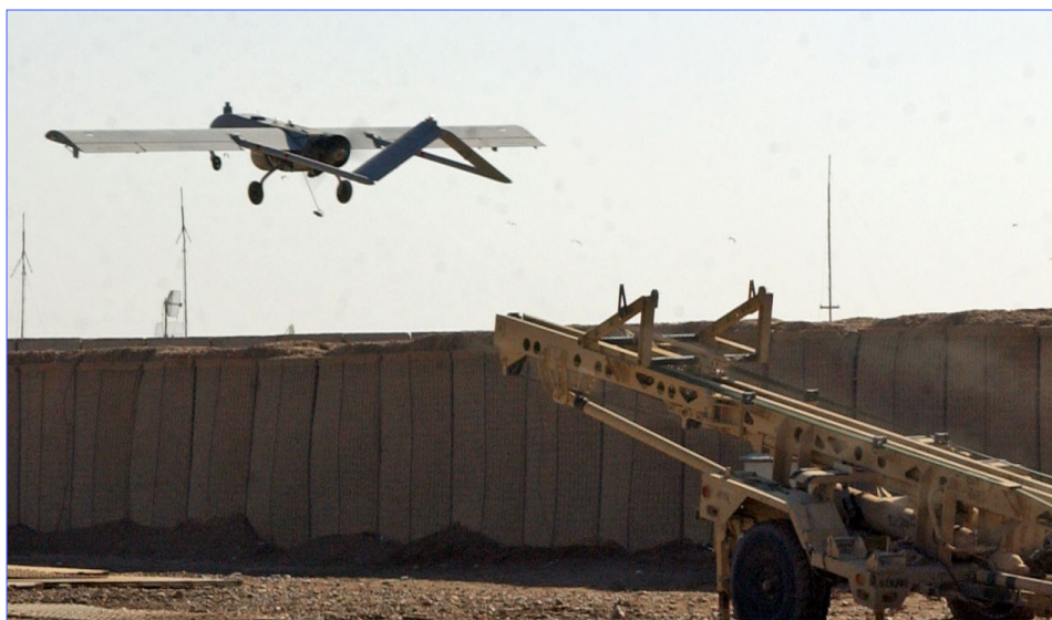
A Shadow UAV is propelled from its launcher to conduct reconnaissance during a training mission.
